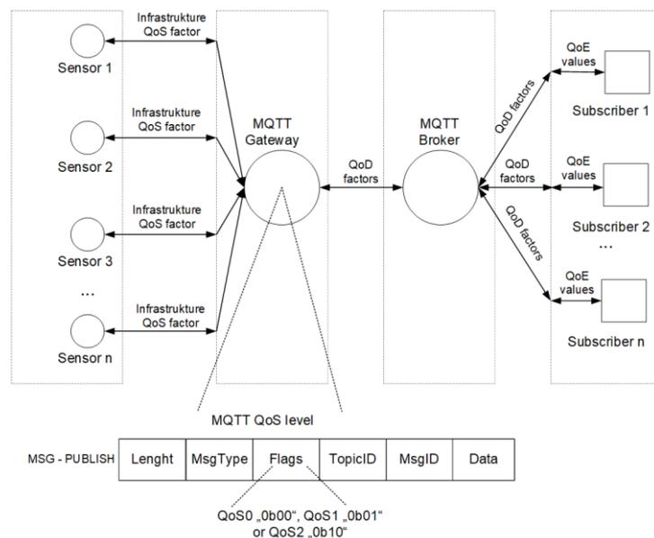
**Fig. 2.** Structure of proposed model for quality-focused parameters monitoring
