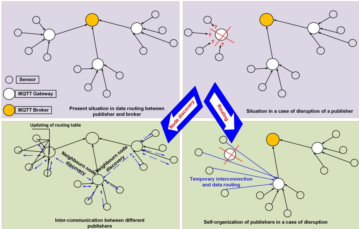
**Fig. 3.** Present situation and proposed solution for WSN-based water distribution system in a case of disruption
