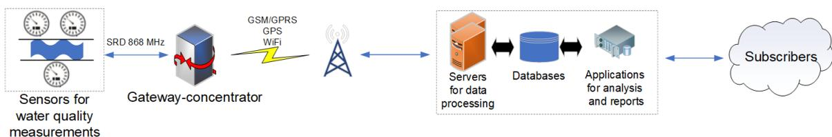
**Fig. 1.** A general structure of WSN-based water distribution system [1]
